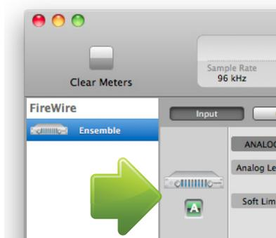
A device icon and ID button is placed adjacent to each row of parameters to identify the hardware unit to which the row belongs. By clicking on the ID button, the corresponding hardware unit’s front panel will illuminate. Each hardware unit is assigned a Peripheral Prefix (A-Z, found in Maestro’s Device Settings tab window) which is displayed on the ID button.
