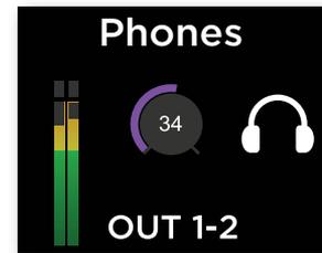
The controller knob operates in parallel with Maestro's headphone control.
